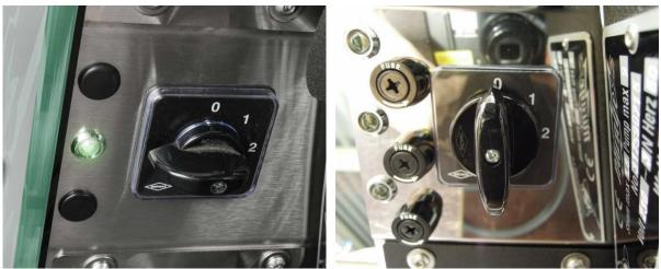
Figure U 1 (left). Showing the mains switch of a Duette with its 3 positions: "0", "1" and "2". Indicator light is lit meaning that heating element is "on". Figure U 2 (right). Mains switch of a (prototype) Triplette with 3 indicator lights and 3 fuses. Mains switch of a Duette high power is identical.
