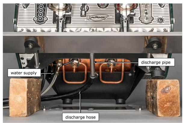
Figure I 3. Mirage Duette tilted backwards by use of 2 wooden blocks and bottom panel removed to show high pressure water supply and discharge hose pushed on discharge pipe. Blocks have dimensions HxWxD = 15x5x20 cm; 6x2x8 inch.
