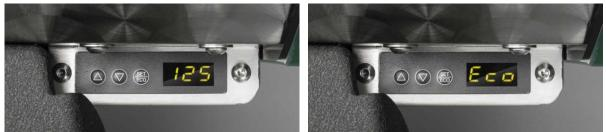
Figure U 4. Showing the steam boiler temperature controller on the lower right side of the machine. Left: temperature in boiler is 125 degrees and heating is "off" - no indicating dot is lit between the 2 left digits. Right: Steam boiler is set at "Eco" temperature (factory set at 70 degrees).
