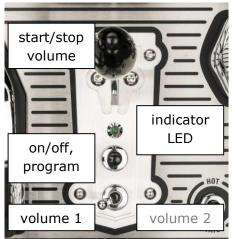
Figure U 3. Functions of a bastone unit of a Mirage. The toggle switch is in the left position, when the bastone is pressed shortly, the brew will automatically stop after preset volume 1 has passed the flow meter.
