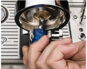
*Figure U 8. Remove dispersion plate from group head.*
