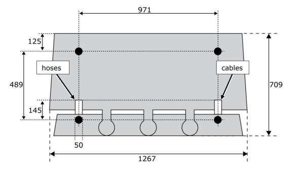
Figure I 1. Footprints of Spirit Duette (top) and Triplette (bottom). Measurements in millimetres.
