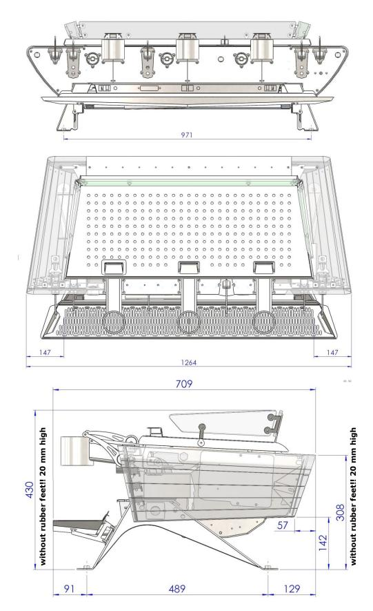
Figure I 3. Measurements of Spirit Triplette. The rubber feet have not been mounted yet, these are 20 mm high and have a diameter of 50 mm.
