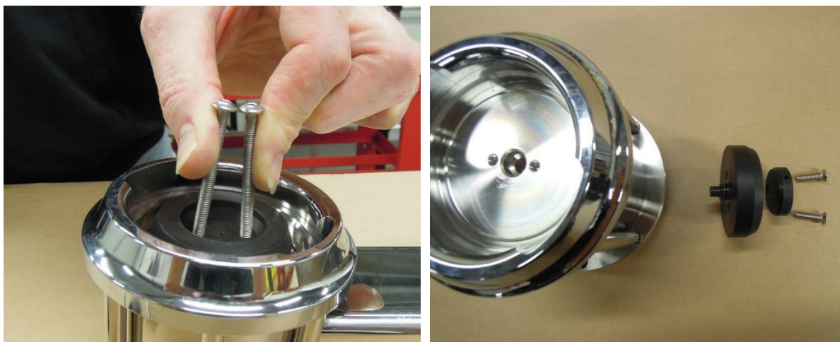
Figure 17. How to remove the dispersion block if it does not come out easily. The picture on the right clearly shows the protrusion on the dispersion block.
