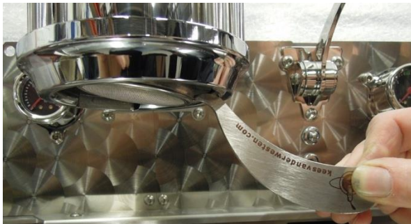
Figure 15 a (left). Pry left and right with screen extractor to remove group screen and group seal.
