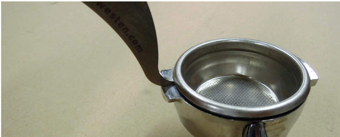
Figure 14. Pry filter basket from filter holder with the group screen extractor.
