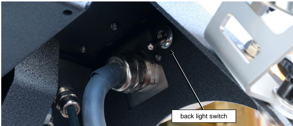
Figure 3. Showing the switch that turns the back LED's on and off (lever pointing down is "off").
