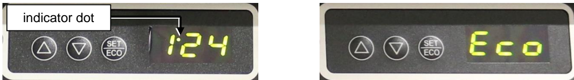
Figure 10. The Störk ST25-Eco controller. (Left) The lit indicator dot signifies that the heating element is activated. (Right) the controller in ECO-mode.
