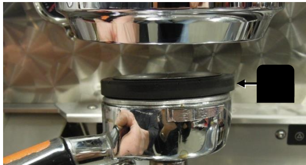
Figure 15 a (left). Pry left and right with screen extractor to remove group screen and group seal.
